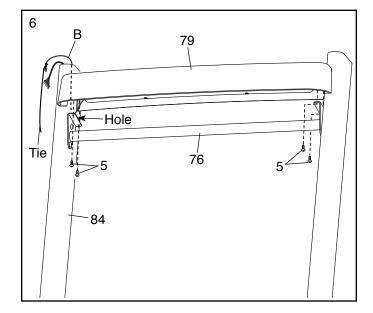
Attach the two Handrails (74) to the Uprights (84) with two of the 5/16" x 2" Screws (2) that you removed in step 3 and two 5/16" Star Washers (8). Do not fully tighten the Screws yet. Be careful not to pinch the Upright Wire (83) or the fan wire (B) on the right side. Position the wires as shown.
