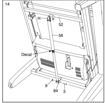
15. Align the upper end of the Storage Latch (56) with the bracket on the Frame (52). Insert a 5/16" x 2 1/4" Bolt (4) through the bracket. This should push a spacer (I) out of the other end. Discard the spacer.
