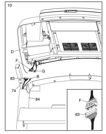
Attach the console assembly (D) to the Handrails (74) with four 5/16" x 2" Screws (2) and four 5/16" Star Washers (8). Start all four Screws, and then tighten them. Be careful not to pinch the wires.
