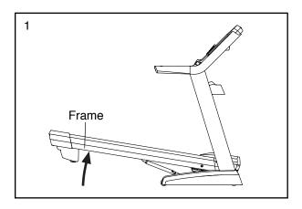
Raise the frame until the storage latch locks in the storage position. CAUTION: Make sure that the storage latch locks.
