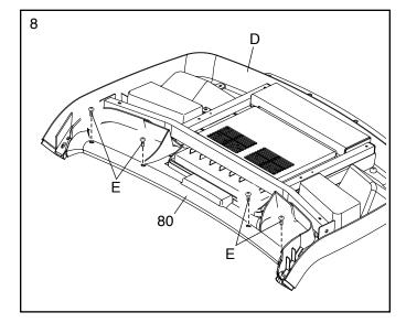
9. IMPORTANT: To avoid damaging the Pulse Crossbar (80), do not use power tools, and do not overtighten the #10 x 3/4" Screws (6) or the 5/16" x 2" Screws (2).
