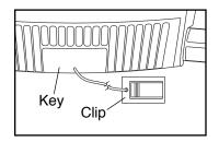
into the console. Note: It may take a minute for the console to be ready for use. IMPORTANT: In an emergency, the key can be pulled from the console, causing the walking belt to slow to a stop. Test the clip by carefully taking a few steps backward; if the key is not pulled from the console, adjust the position of the clip.
